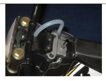
6. Remove the objects from bag X-010 and fix the foot supports using 2 M4x12 hex screws after applying tread lock.
