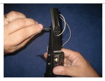
6. Remove from bag X-113 the left top frame ( which has a window to fix a servo in the upper part)and fix it to the tail saver with 2 screw for plastic without tightening too much. PHOTO.
