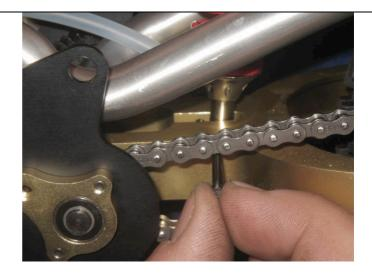
6. 33. Lock the pin with a M4 set screw.
