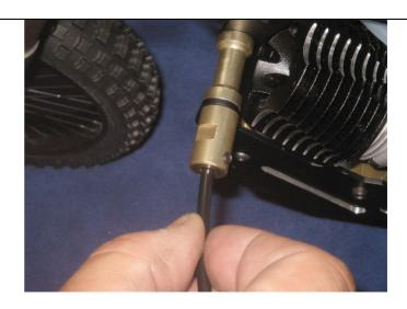
6. 58. Before moving to the next assembling module check the alignment between the rear tire and the rear body shell retaining pin.
