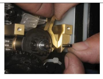
6. 27. Check the brake can move freely
